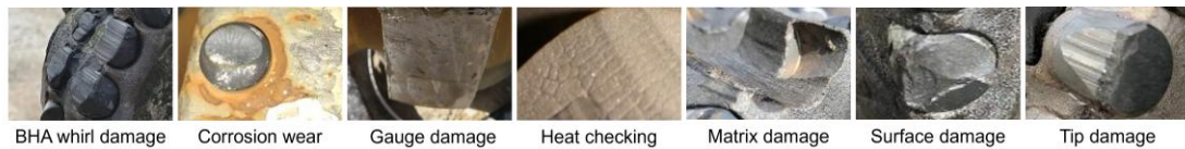
Fig. 1 Representative samples of the seven damage categories in the drill bit damage dataset.
