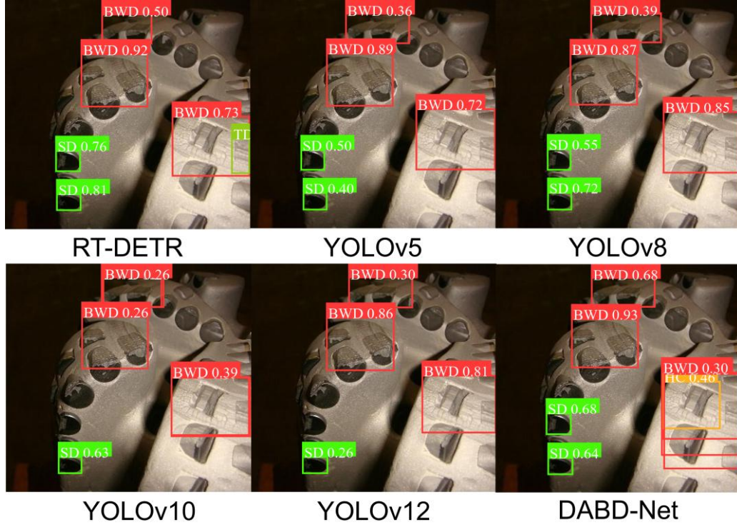
Fig. 11 Comparison of drill bit damage detection results in dim environment
