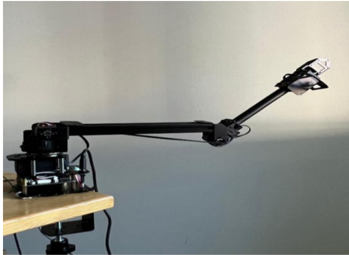
Figure 18. Final position of the robotic arm after execution of PLC-generated joint angle commands.
