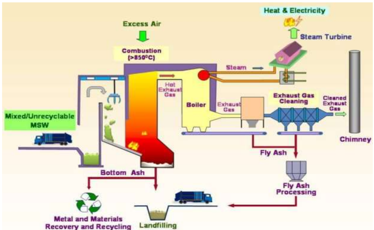
“Fig. 1.” Waste-to-Energy Incineration Process [11].
