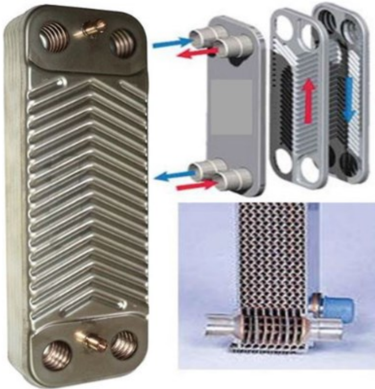
Figure 25 Brazed compact heat exchanger (Kilic, 2021, p. 3908)
