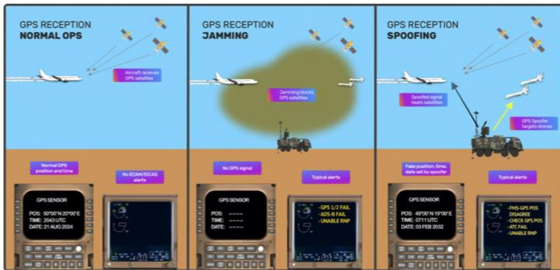
Picture 1. GPS Reception during normal ops, jamming, and spoofing. (OPSGROUP technical guide, 2024)
