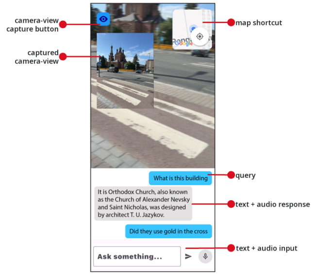
Figure 2: UrbanSearch, the technology probe interface. The interface supports multimodal interaction for situated information seeking in urban space. Users can capture their camera view (top-left) and attach it with a text query, and check their current location in Google Maps through the map shortcut (top-right). Conversational search occurs through the conversational interface (bottom), which accepts text or audio input and returns text + audio responses in a multi-turn dialogue format.
