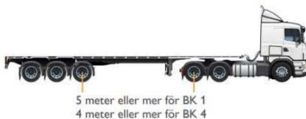
Figure 21. Shows how the distance between the last axle of the tractor unit and the first axle of the semi-trailer is measured. (Transportstyrelsen, 2024)
