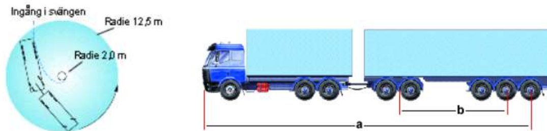
Figure 20. The turning requirement is considered fulfilled if the distance a is not more than 22,5 m and the distance b is not more than 8,15 m. (Transportstyrelsen, 2024)
