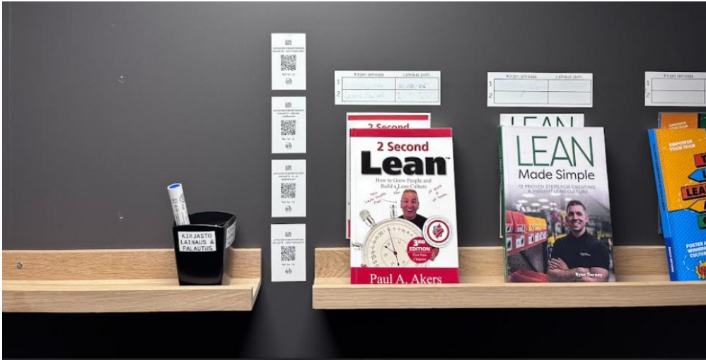
Picture 4. GembaDocs QR-code-only SOPs posted at the point of use (ABB IEC LV Motors Vaasa, 2026d).
