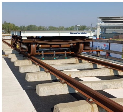
Figure 12: Sleepers, Rail-tracks, and the Test Vehicle (Jansen et al., 2025)
