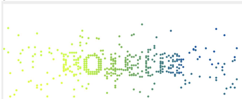
Figure 5 Example of a DotCHA CAPTCHA, each letter must be individually identified (Suzi & Sunghee, 2019).
