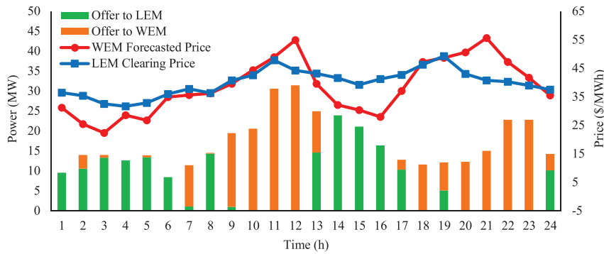
FIGURE 6 Offers of the AG to the DA markets and their energy prices. AG, aggregator; DA, day-ahead.
