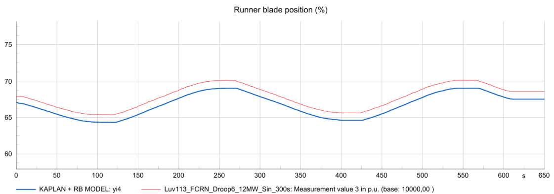
Figure 29. FCR-N sine test 300 seconds: runner blade position (%), measured data (red) and simulated response (blue).
