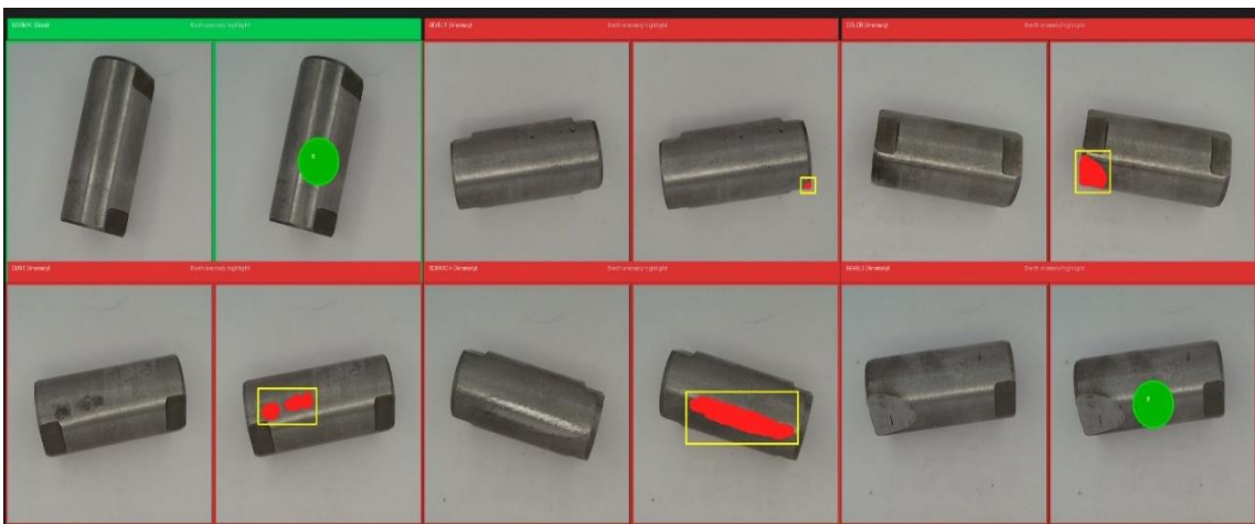
Figure 5. Industrial inspection interface showing side-by-side comparisons of raw component captures against anomaly-mapped results, featuring colour-coded status banners
