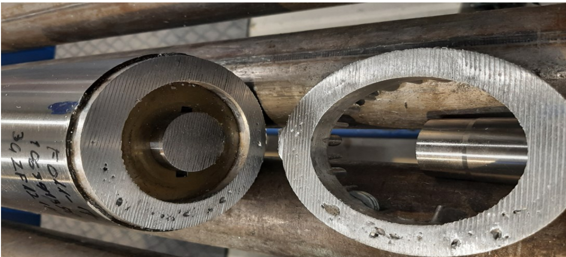
Figure 17. Casting defect found from one of the short circuit rings of studied rotor core 11-17.
