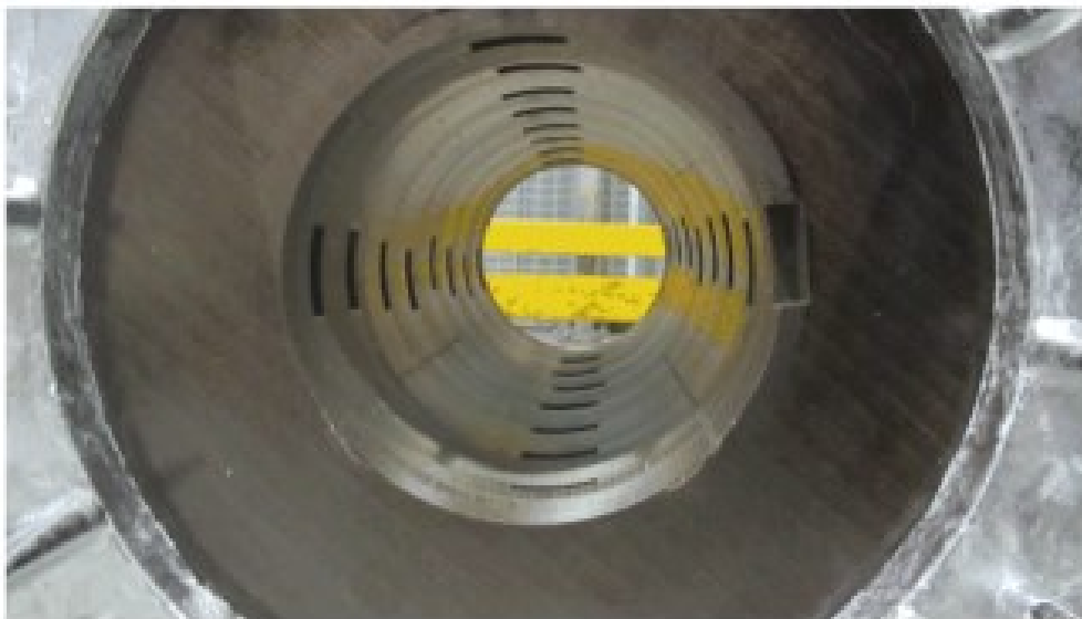
Figure 5. Stacked rotor core when the bundles are turned 90 degrees (Haarala, 2018, p. 3).
