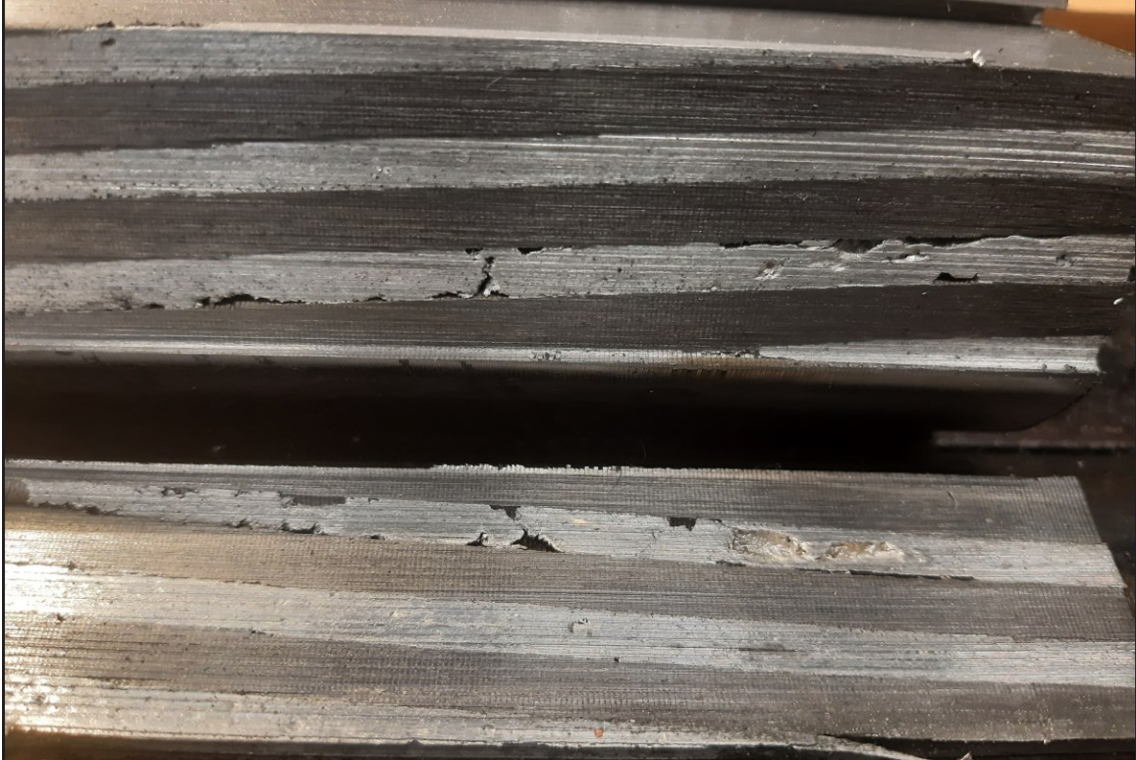
Figure 18. Uneven distribution of aluminum in couple of the slots on studied rotor core 11-17.
