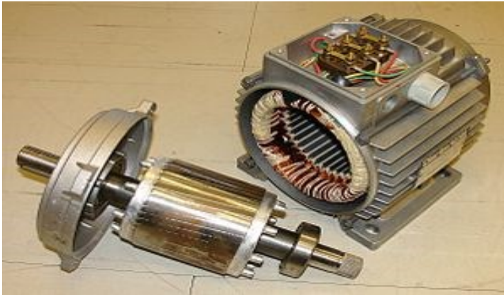
Figure 3. Squirrel-cage rotor. (Zureks 2023).
