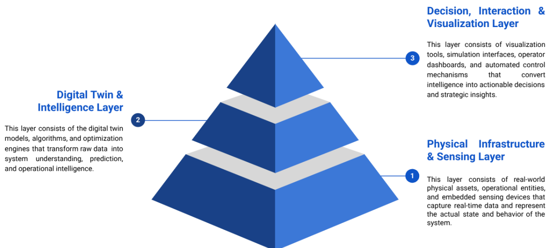
Figure 32. Hierarchical Framework for Digital Twin Integration.
