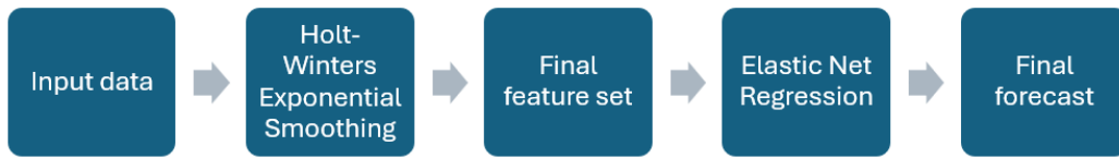
Figure 26 Holt-Winters - Elastic Net Regression hybrid model framework
