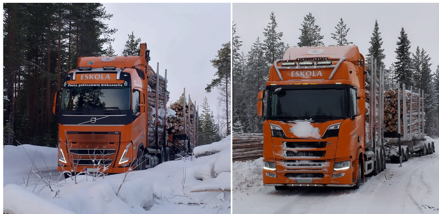
Fig. 1. Liquefied biogas (LBG)-powered (left) and diesel-powered (reference) (right) timber-truck combinations evaluated in this study.
