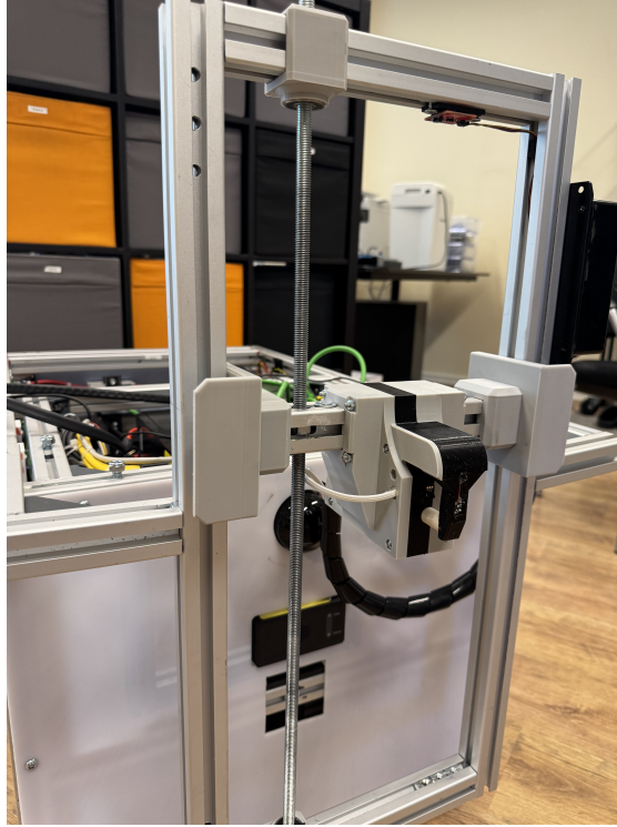
Figure 14. Threaded-rod transmission used to convert motor rotation into linear Z-axis motion.
