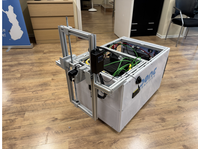
Figure 21. Integrated prototype mounted on the robot platform with hook subsystem and tracking tag.
