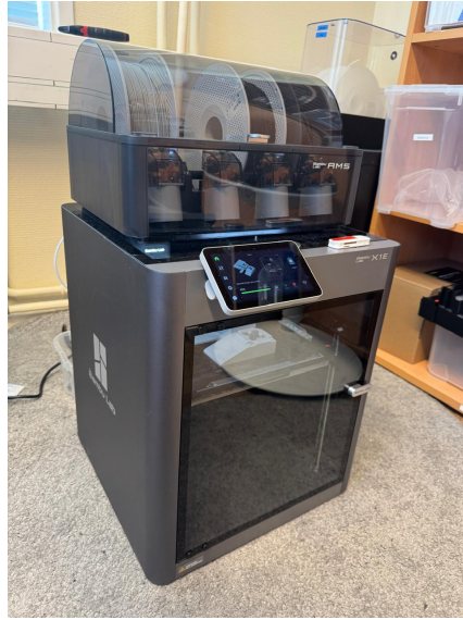
Figure 7. Bambu Lab 3D printer used to manufacture structural and functional components.
