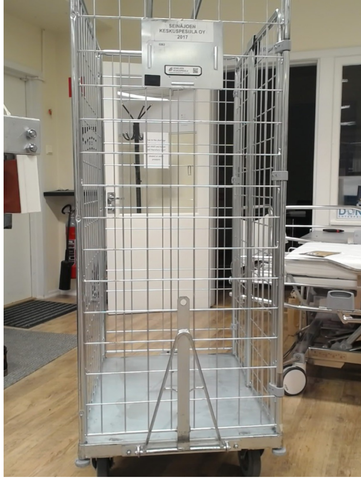
Figure 23. Docking target trolley handle with internal hole geometry used for final visual alignment and hook engagement (source: author's own photograph).
