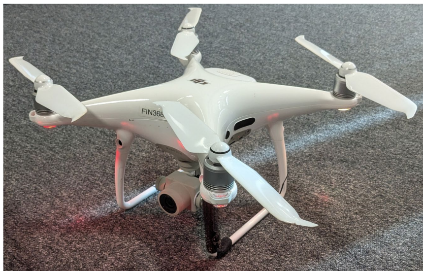
Fig. 3 The DJI Phantom 4 UAV used for collecting the data.
