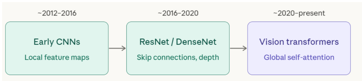
Figure 2. Deep learning architectures for visual defect detection(adapted from Alzubaidi et al. (2021) and Vasan et al. (2024)).
