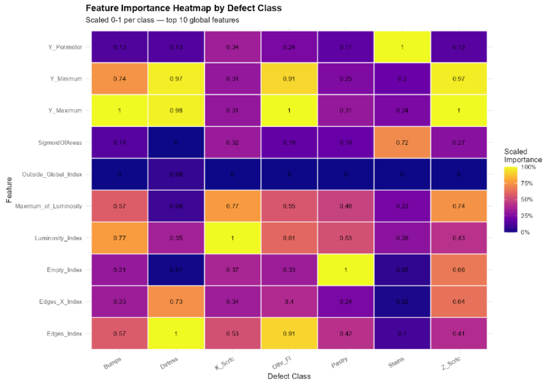
Figure 19. Feature Importance Heatmap by Defect Class (scaled 0-1 per class, top 10 global features). Source: Author's own creation.
