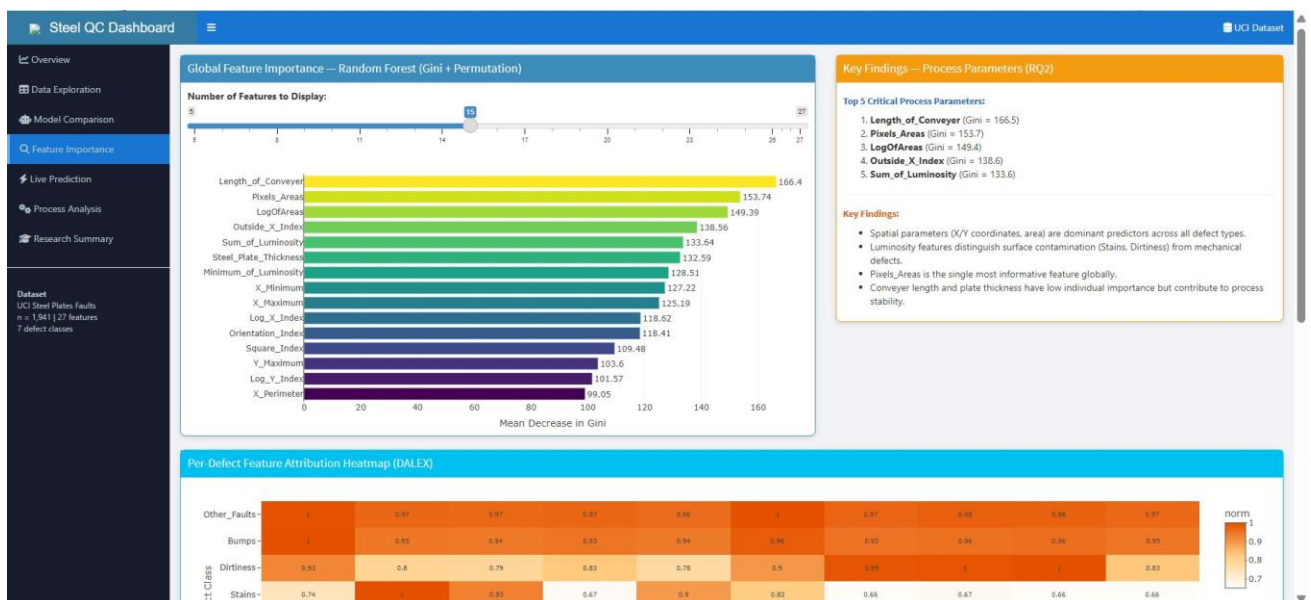
Figure 25. Shiny Dashboard Feature Importance Module with Gini bar chart and DALEX attribution heatmap. Source: Author's own creation.
