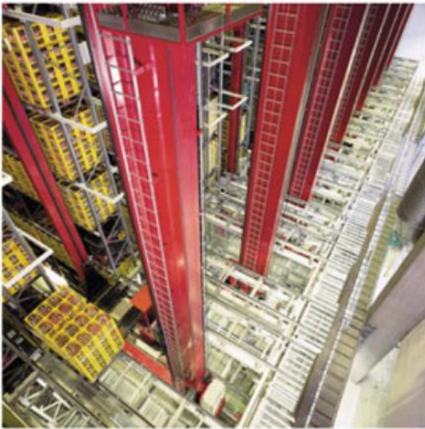
(c) Top view of a person-on-board automated storage and retrieval system (AS/RS)(Vanderlande Industries)
