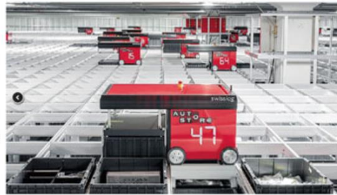
(f) Fully automated warehouse using autonomous vehicles for tote storage and retrieval (Swisslog).
