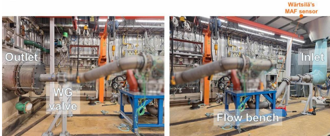
Image 1. Exhaust flow configuration at the GKN Aerospace facility. Air enters via the 'Inlet' (right), passes through the cylinder head mounted on the central test stand (labelled 'Flow bench'), and exits through the 'WG valve' to the 'Outlet' (left). Proprietary components are blurred to maintain confidentiality.
