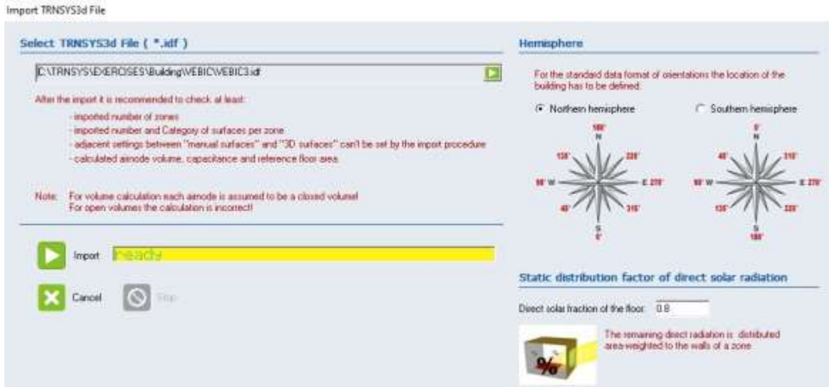
Figure 5. Importing TRNSYS3D file into TRNBuild
