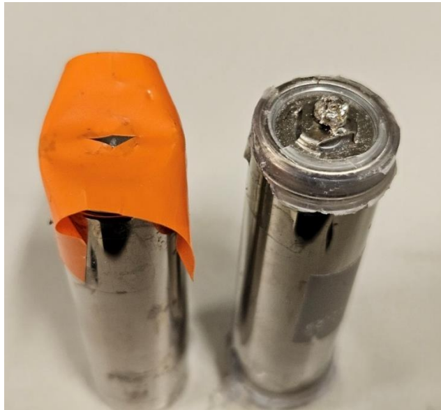
Figure 17. Two different steps to extend and isolate the positive pole from the negative pole
