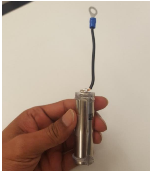
Figure 16. Cable connector technique to extend the positive pole from the negative pole
