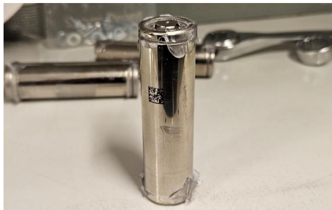
Figure 8. Single cell after dismantling from the 2014 Tesla module
