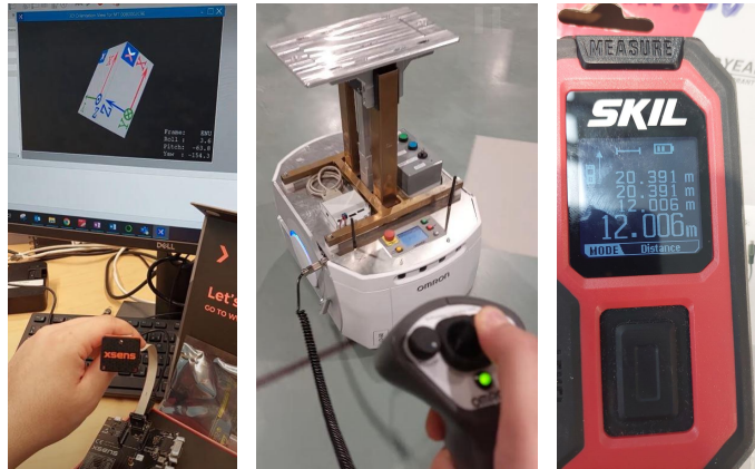
Figure 23. Calibration of IMU, surveying new OMRON map, and LASER-metering the coverage area.
