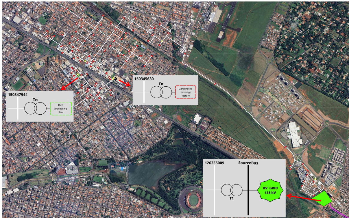
Fig. 3. Feeder ULAE714 region. A rice mill and a carbonated drink industry in highlight [40].
