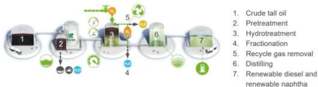
Figure 1. CTO-based renewable fuel production process.
