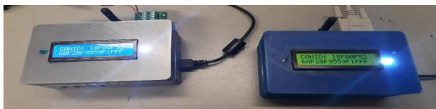
Fig. 7. Wireless Xbee-CAN prototype in 3D printed casing.
