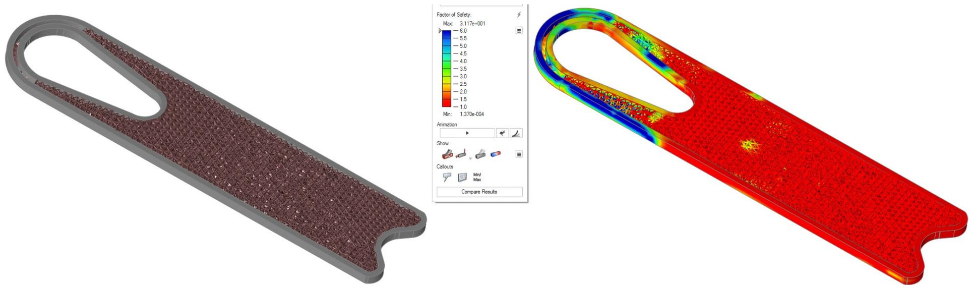
Figure 22. a) Optim 3, Lattice, Mass target – b) FEA
