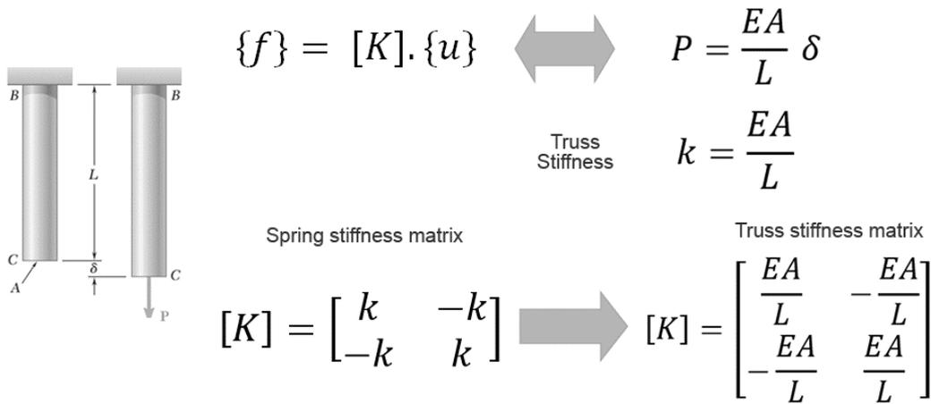
Figure 5. Linear stiffness in FAE analysis
