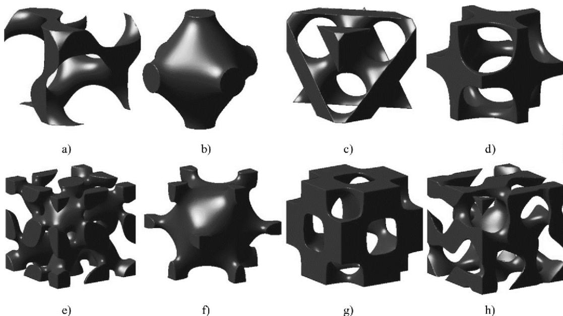
Figure 3. a)Gyroid b)Primitive c)Diamond d)iWP e)Lidinoid f)Neovius g)Octo h)Spilt
