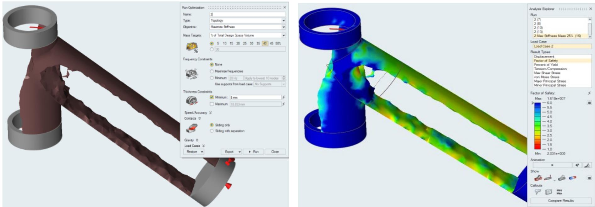
Figure 14. a) Optim 1, Max stiffness, Total mass to 40% – b) FEA
