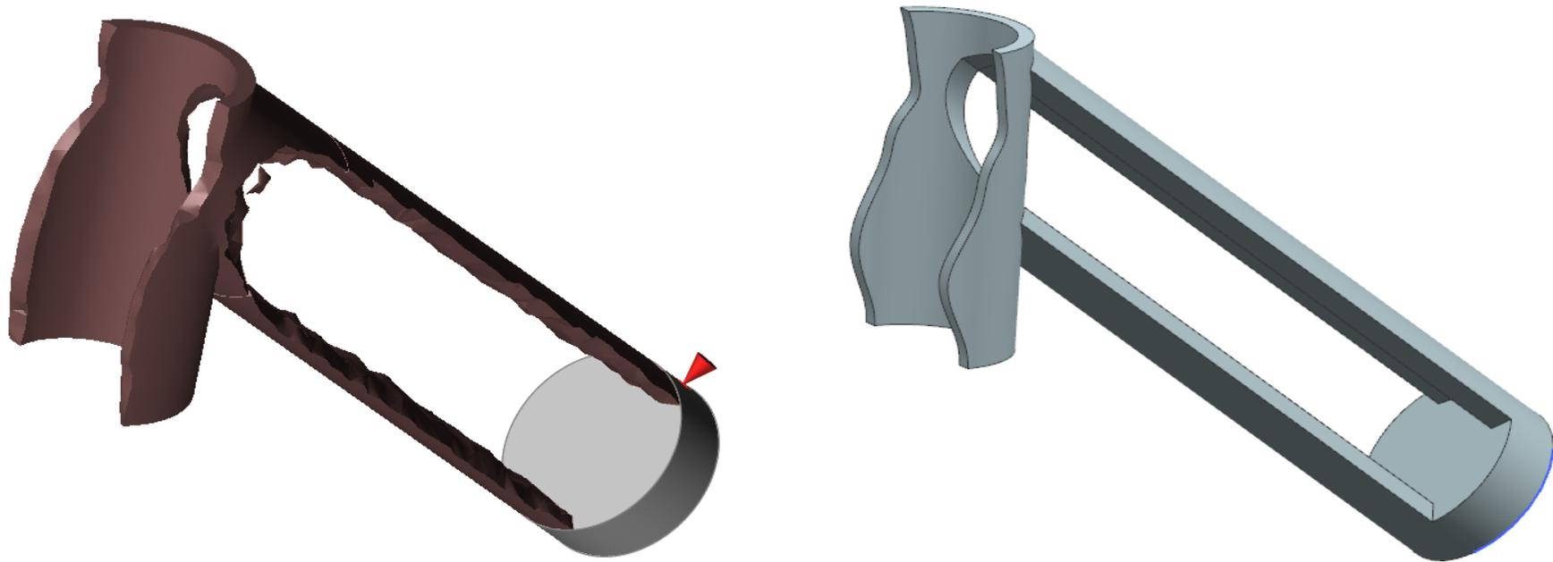
Figure 18. Construction neck part PolyNURBS
