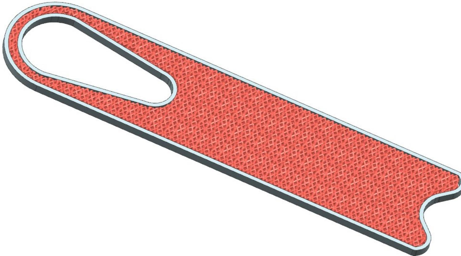
Figure 24. Lattice for platform base with NX
