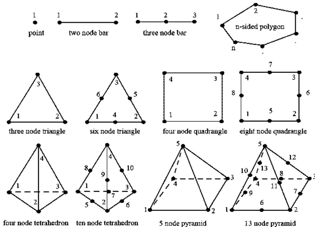
Figure 4. Different types of basic FEA elements
