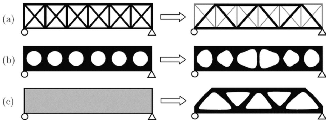
Figure 10. Categories of optimization a) Sizing b) Shape c) Topology
