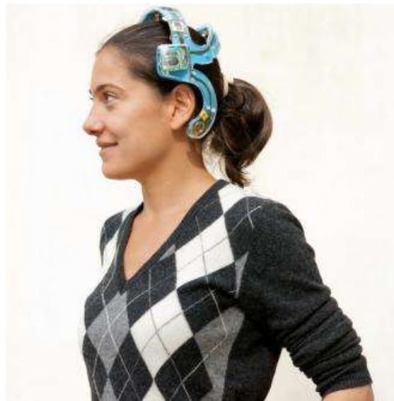
Figure 15. imec's EEG measuring wearable headset.
