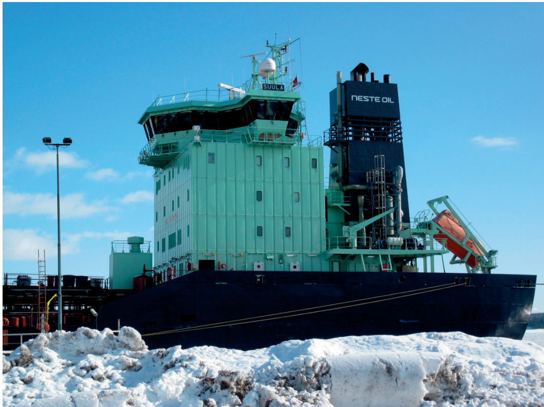
Figure 3-1. Exhaust gas scrubber system installed on board MT Suula. The units are located in front of the blue funnel (Kai Saarinen).
