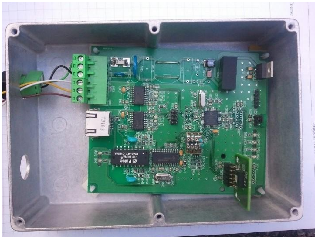
Figure 76. Final anti-sway production board (with Ethernet and 2 Modbus ports).
