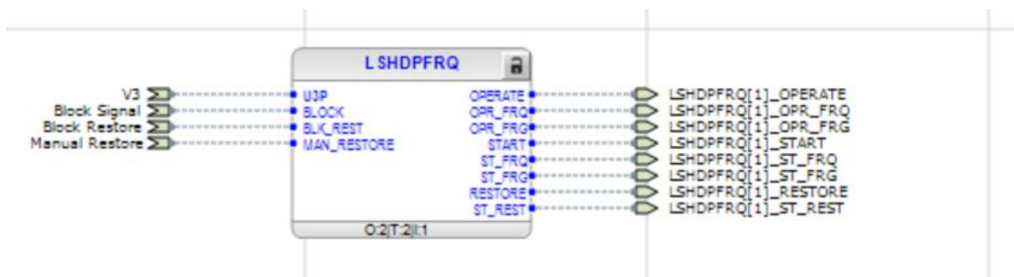
Figure 18- Load shedding and restoration (LSHDPFRQ) function block
