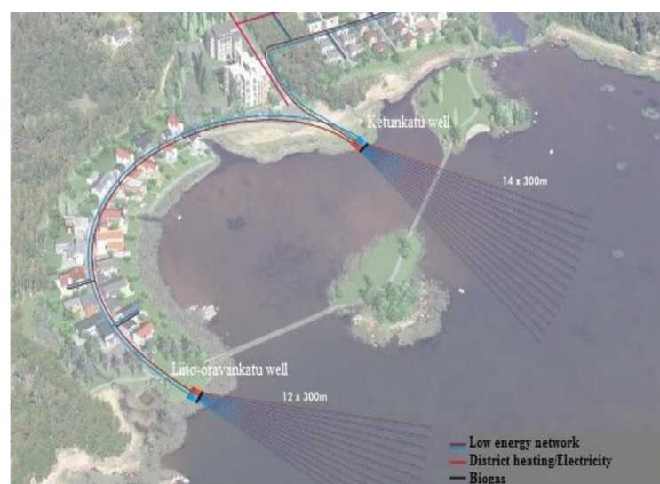
Figure 1. Suvilahti low-energy network sharing heating and cooling for 42 houses (Vaasan Ekolämpö Oy).
