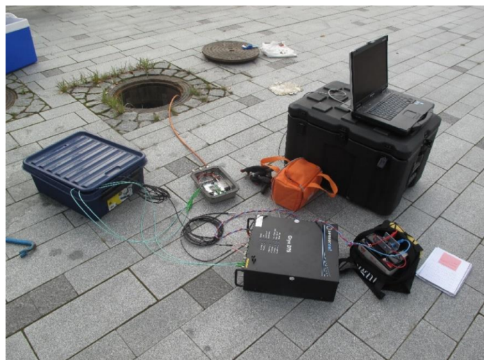
Figure 3. Sensornet Oryx DTS device that can be used even in outdoor conditions.
