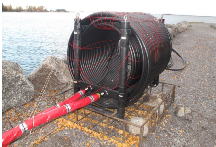
Figure 3. The water heat exchanger that was planned to be installed in Merten Talo is connected to the tubes (of the heat pump in the home), which are insulated. The red wire is the temperature sensors (Picture taken by Anne Mäkiranta during installation process 18 October 2018).
