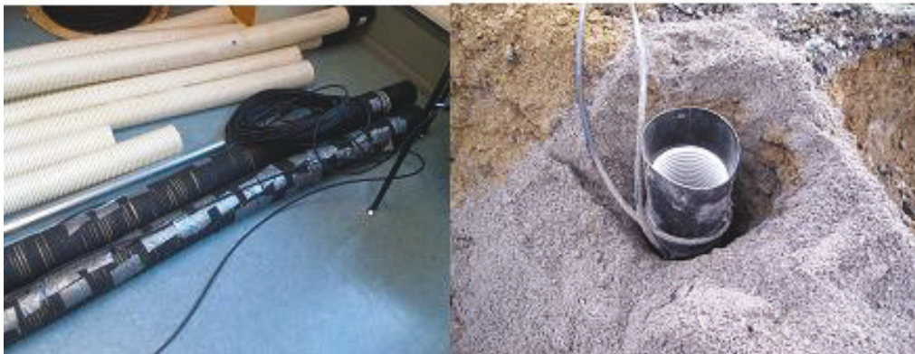
Figure 1. The tubes to measure the soil temperatures.
