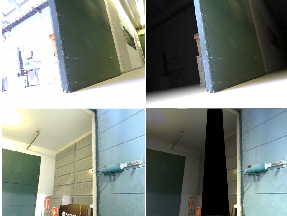
Fig. 3: Synthesized query image samples. Left-hand images have been extracted from the laser scanner data without modification, whereas their right-hand counterparts are after lighting adjustment and addition of 2D occlusion (lower-right image).
