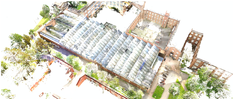
Fig. 1: Overview of the laser-scanned building, acquired by registering the 182 point clouds that consist the 3D dataset.
